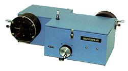
years of accurate and reproducible wavelength positioning. You can use it with the 789A-4 scan controller and software with data acquisition too. Double monochromators are best for applications requiring the lowest levels of scattered or stray light. Applications include source and detector standardization, radiometry, Raman and photoluminescence.
