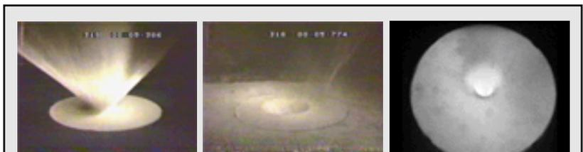
*Still photos from a high-speed image sequence (one millisecond between each frame) of an impact by a copper sphere traveling at 4.5 km/sec into porous pumice. A bright "flash" is a high temperature plume resembling a Roman candle that shoots out of the hole created as the projectile penetrates into the target. The ejecta curtain resembles a funnel. These images courtesy of the NASA Deep Impact web site and Dr. P. Schultz, Professor of Geophysics with Brown University.*
