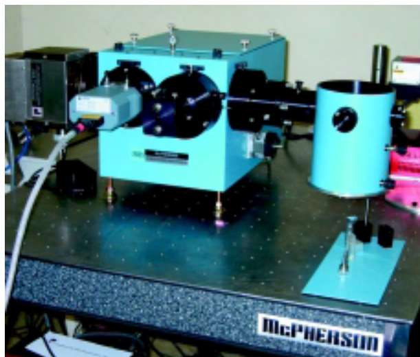
Raman Workstation shown with 50mW DPSS 532nm laser, macro sample chamber, 350mm f/4.8 spectrometer, cooled photomultiplier tube housing and CCD array detector.
