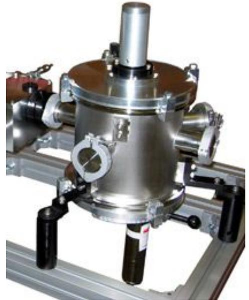
The sample chamber allows (goniometric) independent positioning of the sample and detector. Set the angle even while under vacuum. Set the detector angle from < 15 to 180 degrees. Adjust sample angle from 0 degrees to 60 degrees. Angular scales read out in degrees. Options exist for three- and five-position sample mounts. The three-position mount is a better choice when reflection measurements are required.
