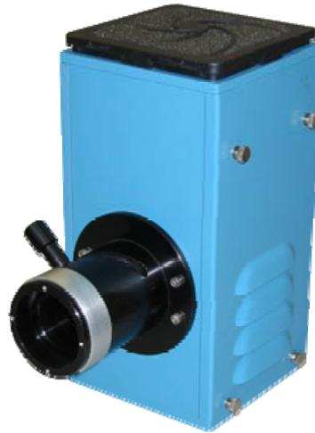
**Operates a variety of sources | Rear reflector | Forced air cooling | Fits to McPherson 5" Slits**
